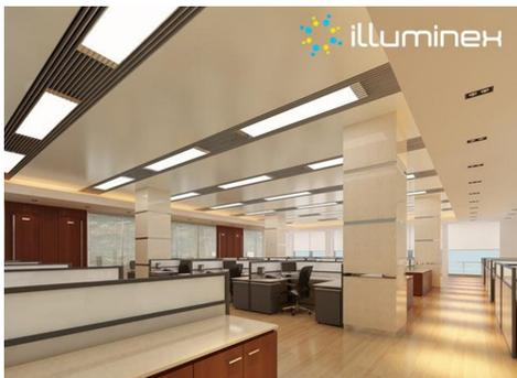
Individual LED's are very small and don't put out much light on their own, but are typically combined together to make lighting fixtures which put out light levels similar to other sources and are flexible enough to mimic the shapes of these sources as well. LED fixtures
